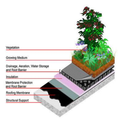
The above diagram demonstrates the different levels in a green roof
