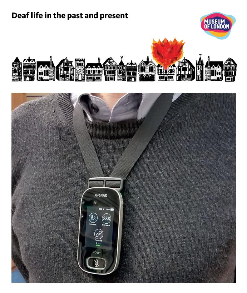
**Radio aids** pick up a speaker's voice and transmit it to receivers on hearing aids and cochlear implants.
